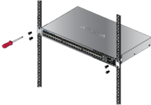
Figure 3-5: Inserting the Switch into the Rack
