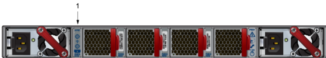
Figure 14: Earth Grounding Pad Sockets for Models without Management Ports on the Rear Panel
