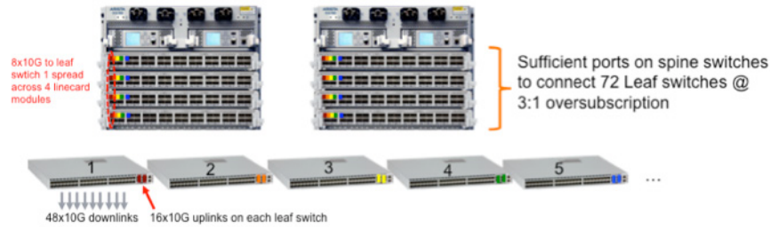
Figure 8: Final expansion of spine in a scale-out design: add a fourth linecard module to each Arista 7504
