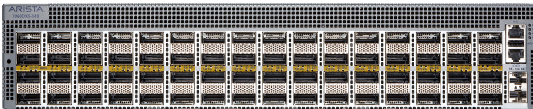
Figure 11: Arista 7060DX5-64S: 64 x 400GbE QSFP-DD ports, 2 SFP+ ports
